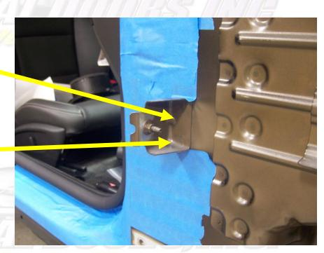
After making sure you have all the marks you need in case the door moves during installation, you can remove the factory door hinges. After removing the factory hinges, you can install the new VDI hinge. You will then be able to raise the door and Install the shock.
