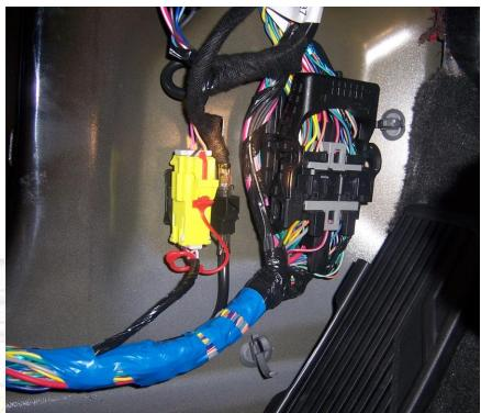
On the passenger's side the wire re-routing will be similar to the Driver's side.
