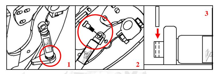
Hint\* (You will need a helper to hold the door). (Slip the bottom shock end into the spherical bearing (1). Using a 1/4 Allen wrench, tighten the shoulder bolt into the swing arm (2). After the shock is installed secure it by installing the pin in the bottom shock end (3).
