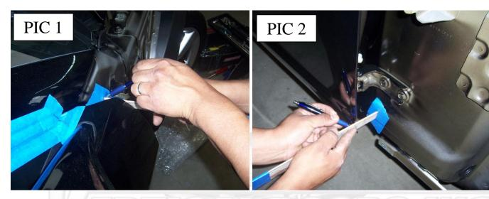
You will have to remove one of the fender brackets. To remove it drill out the 2 spot welds. This will allow a clean removal of the bracket
